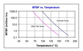
As can be seen from the MTBF numbers above, the predicted failure rate is still above 1 million hours, even at operating temperatures up to  $+130^{\circ}$  C (corresponding to channel temperatures of  $+160^{\circ}$  C). Also note that these MTBF estimates are a lower bound as the accelerated testing never resulted in 50% failures.
